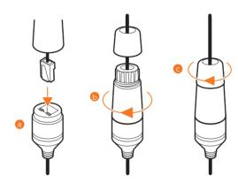
NOTE: When using the waterproof cap, crimp the RJ45 connector after passing the cable through the waterproof cap.
