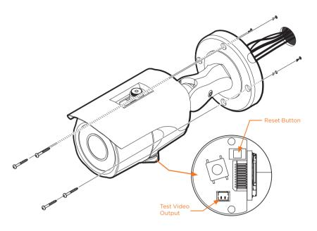
**Resetting the camera:** To reset the camera, use the tip of a paper clip or a pencil and press the reset button. Pressing the button for five (5) seconds will initiate a camera-wide reset of all the settings, including network settings.
