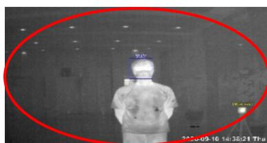
The recommended location for the Blackbody installation: The Blackbody cannot be installed in a crowded location. Install the Blackbody within the red ellipse marked within the image on the left. This is the best location for on-site constant auto-calibration for accurate temperature measurements ( $\pm 0.36^{\circ}\text{F}/0.2^{\circ}\text{C}$ ).
